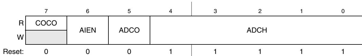
Figure 12-4. Status and Control Register (ADCSC1)
